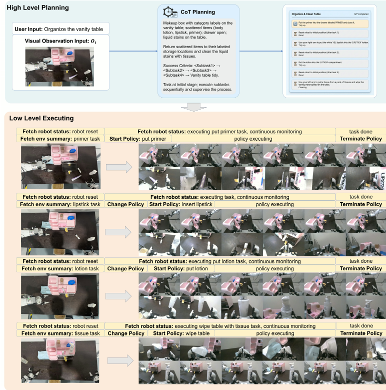
Fig. 5: Long-horizon task execution with agent orchestration. The same VLM-based agent plans over the vanity table tidying task and dynamically composes independent forward policy checkpoints (primer placement, lipstick insertion, lotion placement and tissue wipe), invoking re-planning when needed.
