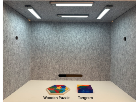
Fig. 1: Physical setup used for data collection. Tangram blocks (Task 1) and wooden puzzle blocks (Task 2) are placed on the table inside a small workspace enclosed by gray walls. Four LED lights are attached to the ceiling wall to provide consistent illumination.
