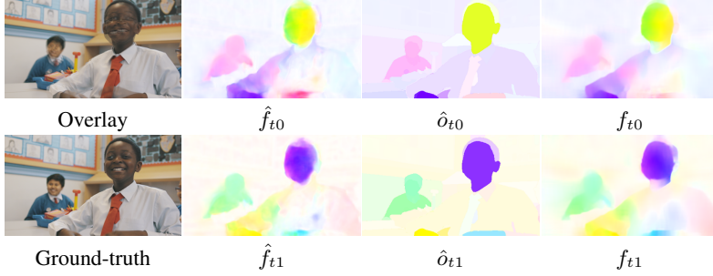
Fig. 4: Visualization of the predicted pixel-level flows \hat{f}_{t0} and \hat{f}_{t1} , pseudo object-level flows \hat{o}_{t0} and \hat{o}_{t1} and pseudo flows f_{t0} and f_{t1} . It shows that object-level optical flows provide useful prior knowledge for suppressing erroneous motion patterns from pseudo-labels, particularly in regions involving large motion, occlusions, and motion boundaries ( See the moving head and hands ).
