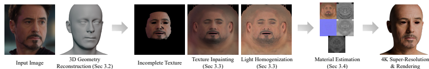
Fig. 2: Overview of our high-fidelity 3D avatar reconstruction pipeline. From a single image, we recover 3D geometry and an incomplete texture map, then repair and homogenize it for illumination. We subsequently predict PBR maps (albedo, roughness, specular, normal) and displacement, enabling photorealistic 4K rendering.
